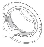
Foreign metal substances in your machine can cause rust stains. In such cases: Clean the drum with a stainless steel cleaning agent. Never use steel wool or wire wool.
